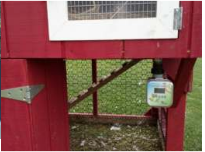
solar water timer converted to switch lights
